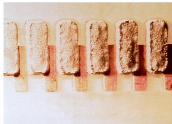
Offset printing of solder paste on printed circuit board pads.
